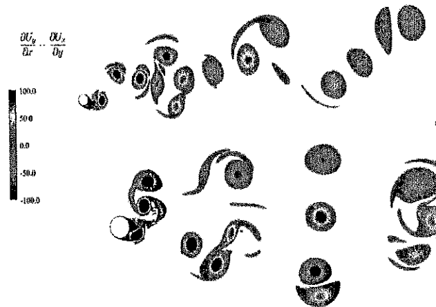
Figure 5. A computed VIV pattern behind the two cylinders
